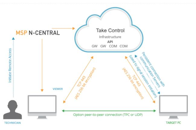
The ports identified in the tables below must be accessible for Take Control (MSP Anywhere) remote control connections.
